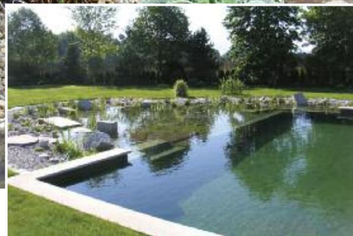
This pool by BioNova Natural Pools features fully biological filtration with local marsh plants growing in the regeneration zone. Except for a small pump, no chemicals or other devices are used at all. Rocks and small boulders enhance this natural setting.
